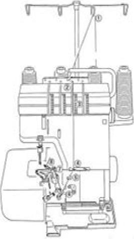
Place the spool of thread on the spool pin second from the right.
