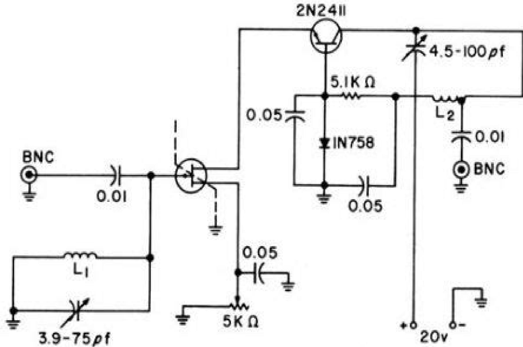
$L_1, L_2$  18 turns B&W 3004 Minductor;  $L_2$  tapped 1 3/4 turns from ground.
