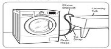
Clip the end of the hose into the elbow bracket. Hang the end of the drain hose over the side of the laundry tub. Use tie strap to secure the drain hose in place.
