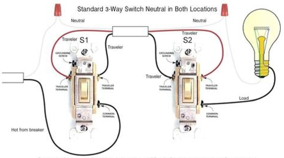
On a standard 3-way switch there are 3 terminals and a ground, 2 Traveller Terminals that are brass and 1 Common terminal
