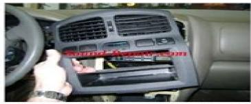
Step 5: Remove 4 screws securing radio to vehicle.
