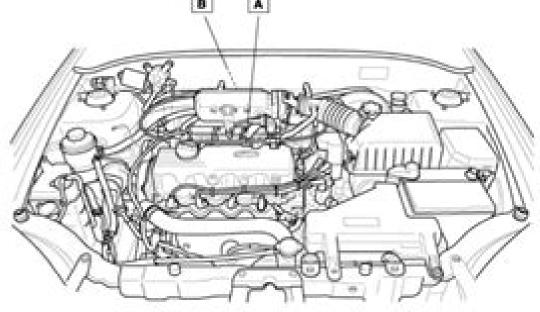
A Positive Crankcase Ventilation Valve (PCV valve)
