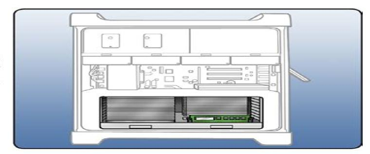
2 Press down and release 2 latches on front of processor tray.
