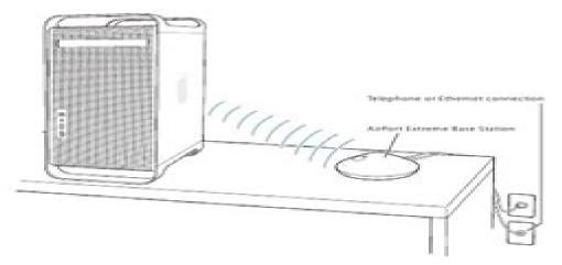
Important: Several kinds of objects placed near the computer can cause interference. See the instructions that come with an AirPort Extreme Card or AirPort Extreme Base Station to learn about avoiding interference. For more information, go to AppleCare Support at www.apple.com/support.
