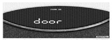
If any other active warnings including "GATE", "GLASS", or "LOWASH" are present, they will be shown in the VF display and will also continue to cycle. If the vehicle is moving, three single chimes will occur (One chime for each complete display cycle (three cycles total). After this, the display will continue to cycle only (no chimes).
