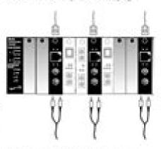
The AutoCross\*\* feature allows either straight-through or crossover twisted-pair copper cable to be used when connecting the C/E-TX-SX-02 to a 10/1008ASE-TX device.
