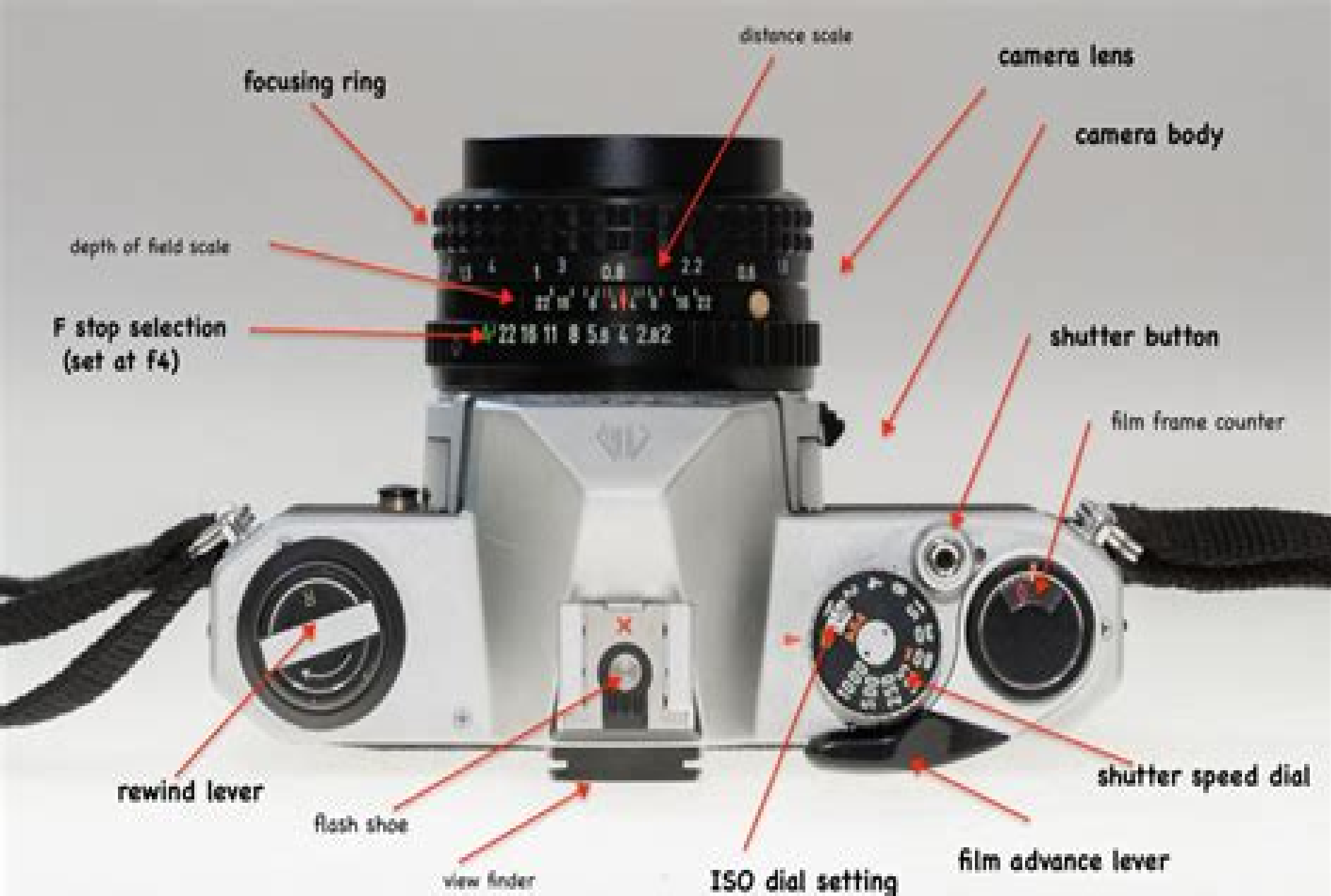
top view 35mm SLR mechanical camera
