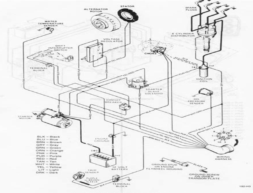
Engine Electrical System Wiring Diagram
