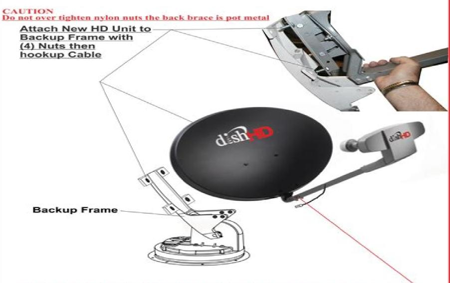
Unit held in Open Position by a small Pin, Remove after Installation is Complete.
