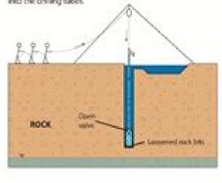
(C) The bit is lifted as the crew pulls again. The valve closes, pushing up the water column inside the hollow tubes. Water and sediments are expelled through the mouth, falling into a decarter. Water in the decanter may flow back into the hole, while sediments remain outside.
