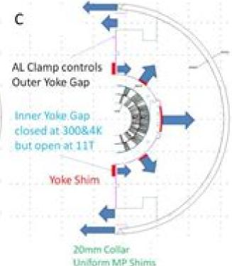
The 20-mm width is the minimal collar width determined by stress limits in the collar and key materials.
