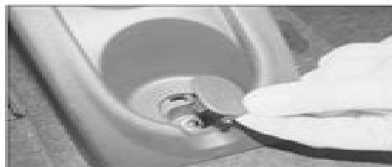
26.5 Extract the trim moulding and undo the console rear retaining nut
