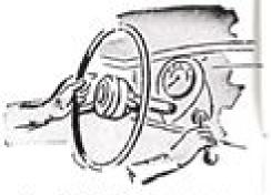
instruments, and accessories. Parking lights operate by rotating knob to "S" position—also controls instrument light. Turning the knob to "H" will turn headlights on and front parking lights off. A map light switch is located under dash panel, to right of the cigarette lighter.
