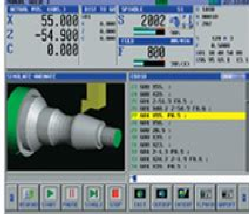
Example of fix programming cycles for turning operations
