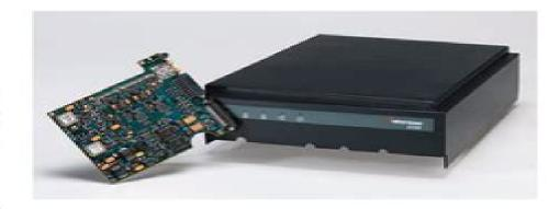
Intellitag 500 reader/ programmer board sets are offered for integration into radio frequency identification (RFID) solutions requiring read range, multitag sort, read/ write, and memory capacity not provided by older, less flexible proximity technology. The flored reader/ programmer board set is designed as an option to the Intermec 2100 Universal Access Point (UAP), but it may be integrated into other microcontroller-based systems.
