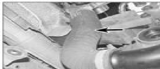
13.9 Slacken the clamps and remove the charge air pipe (arrowed) from the turbocharger
