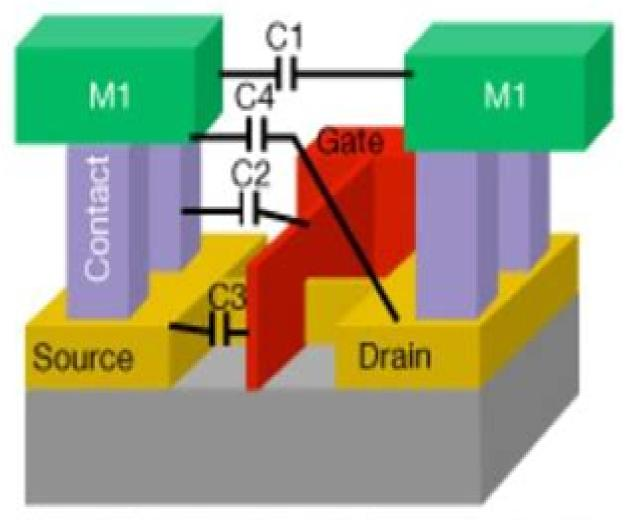
C1: S contact to D contact C3: Gate to S/D diffusion
