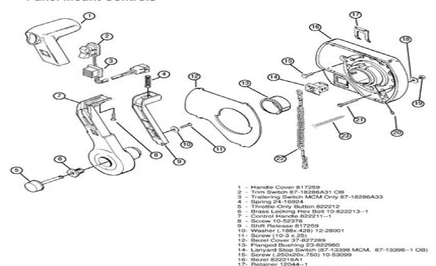
18- Washer (.281x.734x.063) 12-69057 19- Nut (.281x.734x.0) 11-814101 20- Friction Screw 10-824831
