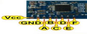
Close the two pads with a drop of solder to enable SLIM mode
