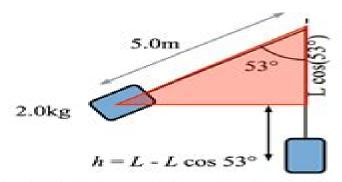
We can find the height of the pendulum bob relative to the bottom of its swing by using trigonometry. The length of the short side of the triangle (shown in red) is  $L \cos 53^\circ$ . The height b is the full length L less this leg of the triangle.
