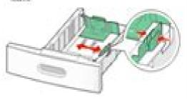
Untiet the length guide, repursor the tanget-guide talons and as shown, and slide the guide to the correct position for the puper size being leaded.
