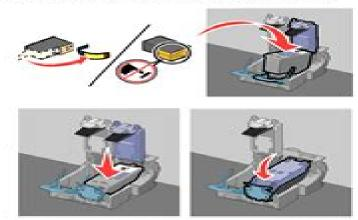
Warning—Potential Damage: Do not touch the gold contact area on the back or the metal nozzles on the bottom of the cartridge.
