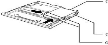
Load the paper into the Cassette with the print side facing DOWN.
