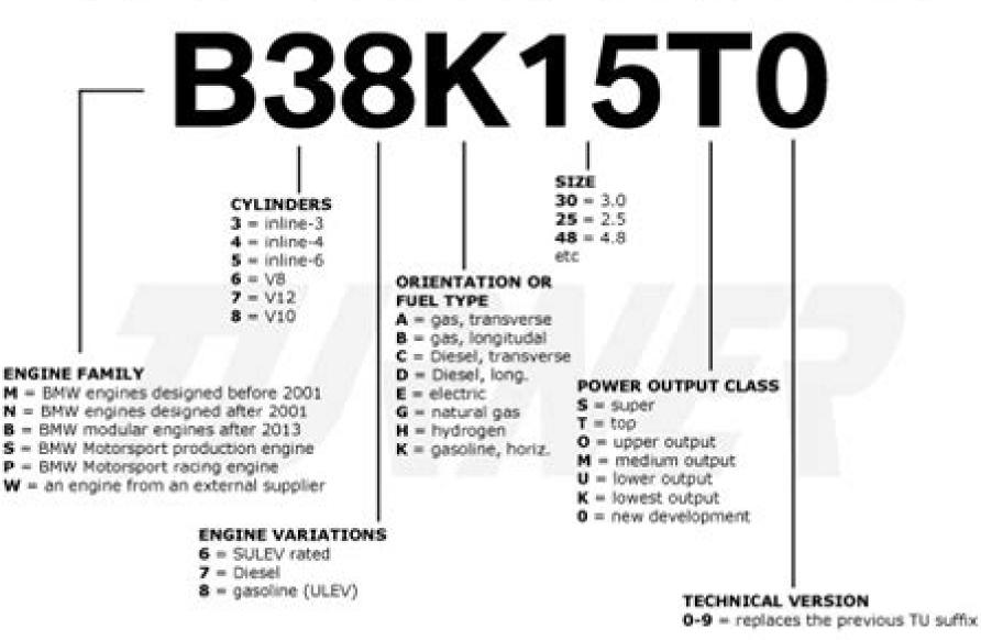
B38K15T0 = modular engine / 3-cylinder / 8th design / horizontal-mounted gasoline fuel / 1.5 liter / Top output / original variation
