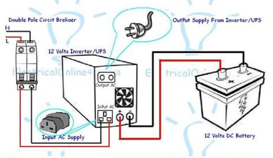
UPS/Inverter battery connection diagram Or How to connect Battery to Inverter/UPS Diagram. ElectricalOnline4u.com
