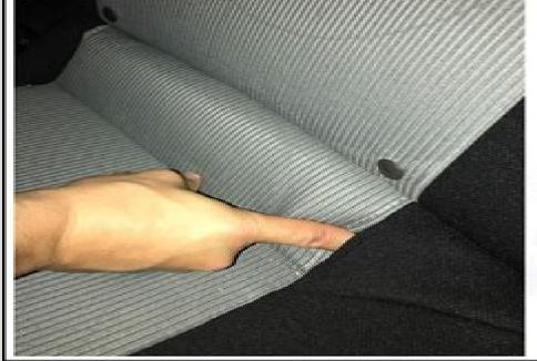
Left: The hand shown here is pointing to the slit provided in the seatback for easy access to the lower anchors.
