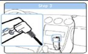
Plag the GPS receiver into the GPS-port and place it in clear view of the sky.
