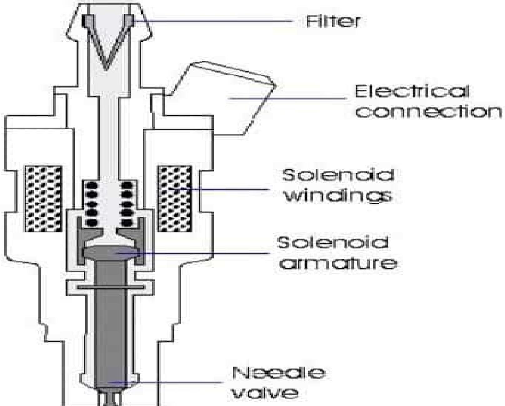
Fig. Electronic Fuel Injector
