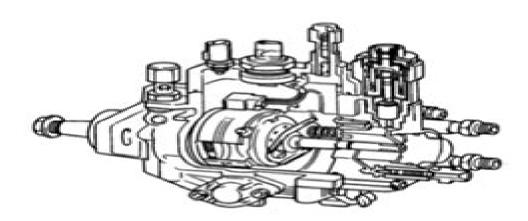
NOTE: Some of the components of the ECD-V5 injection pump system are very similar in design and operation to those of the NP-VE4 injection pump system. Therefore this lesson only describes the components which are new or operate in a different way to those in the NP-VE4 injection pump system.
