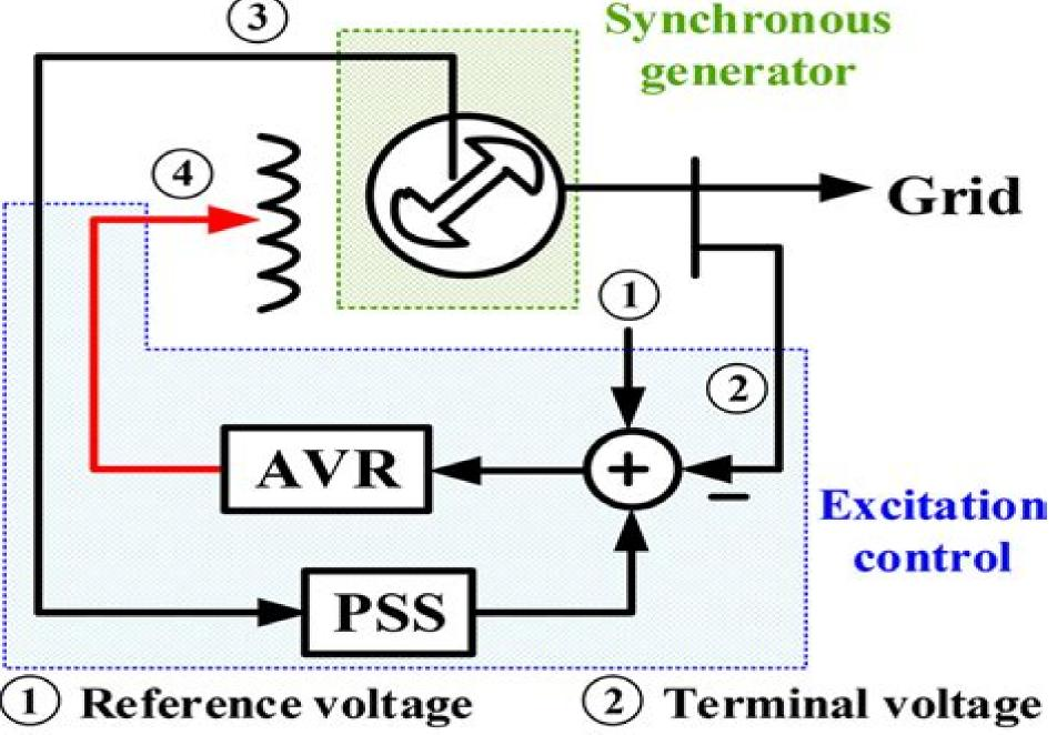
3 Rotor speed deviation 4 Field voltage
