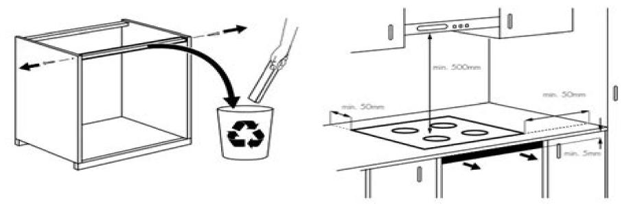
Make sure that a ventilation space of 5mm directly below the benchtop is included in the installation and kept the during use of the appliance. The warranty does not cover functional failures caused by the lack of an adequate ventilation space.
