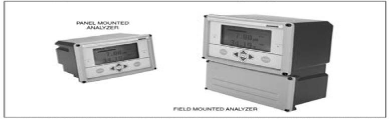
This microprocessor-based, line-powered intelligent analyzer, when used with compatible Foxboro DolpHin<sup>TM</sup> PH10 and ORP10, 871A, 871PH, or EP460 Series pH and ORP Sensors, provides high accuracy measurement of pH, ORP, or ISE. Fortions include measurement display, dual analog outputs, dual relay contacts, and an RS-232 Serial Port for remote configuration. A human interface guides the user through intuitive, menu-driven configuration, status, and troubleshooting procedures.
