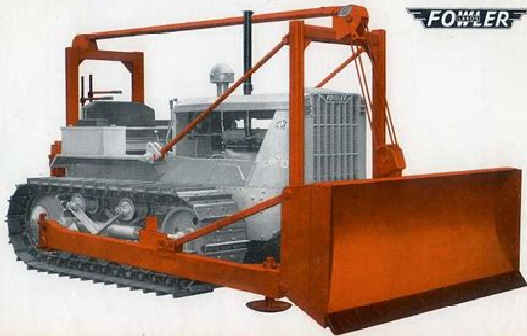
FOWLER CHALLENGER 3 DIESEL CRAWLER TRACTOR with BLAW KNOX CABLE BULLDOZER
