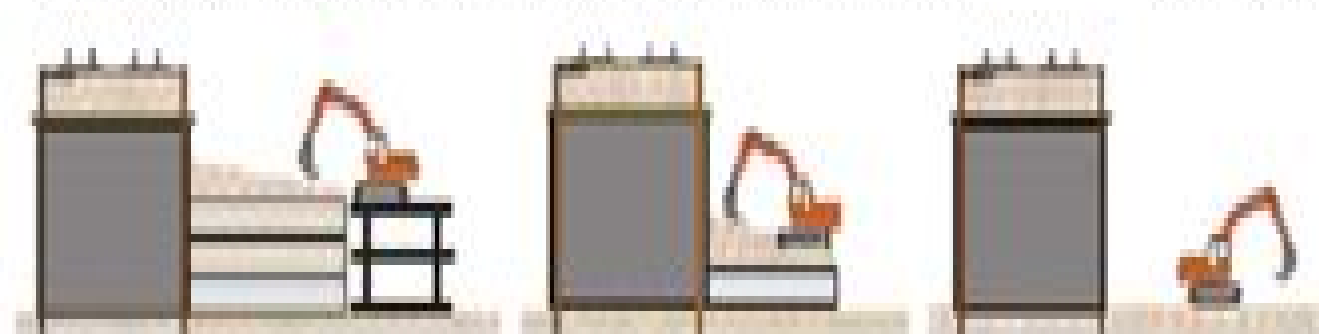
(e) Removed guide boxes and soil
