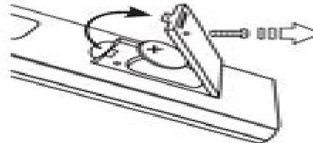
Remove the original battery from the battery compartment and install a new (CR2025) battery with the "+" side facing up as shown in the illustration. Then put the battery cover and screw back to its original place.
