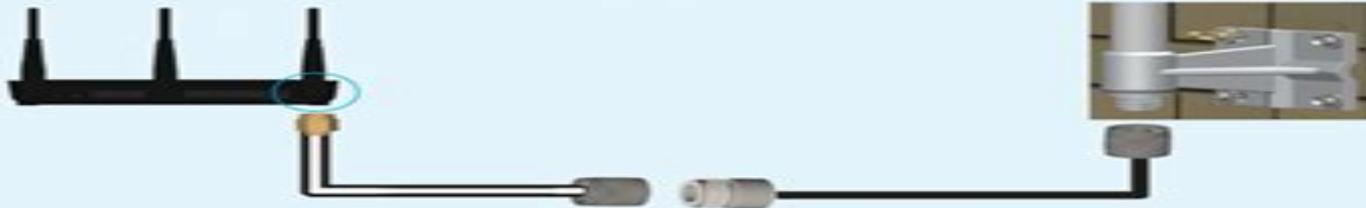
A. Remove the antenna from the HD-45R and affix the small gold end to the antenna port connector
