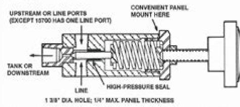
The configuration also makes the control settings virtually unaffected by downstream outlet pressure. This enables the valves to be also used for back pressure control (upstream pressure controller) or as a sequence (priority pressure) valve.
