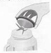
Twist collar onto jar. Be sure to engage threads properly and securely. Turn assembled jar right. side so.
