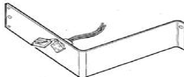
Fig. 2. Proper Installation of Female Receptacle Plug
