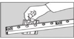
If your wall is uneven use shims between the rail and the wall to make sure the rail is flush.
