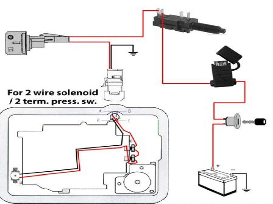
700R4 non-computer TCC wiring USING 4TH & 4/3 PRESSURE SWITCHES
