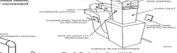
Fig. 5. Typical upflow HVAC system.
