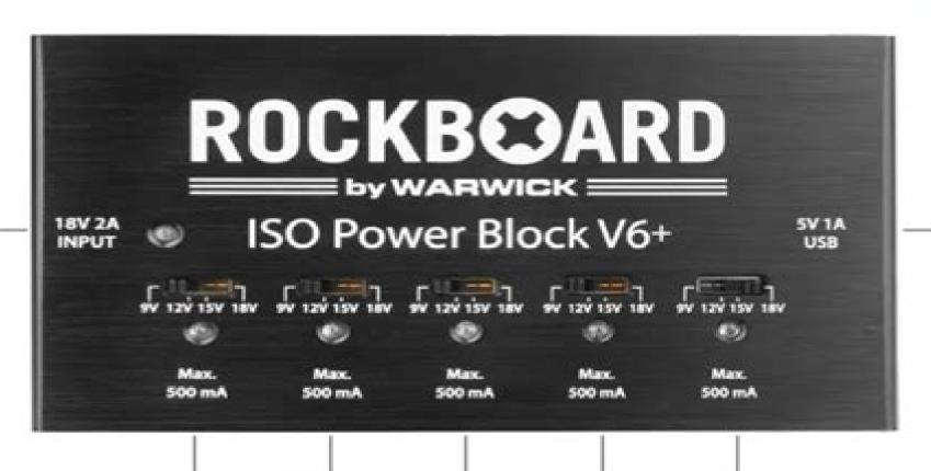
5 x switchable slots with 9V DC / 12V DC / 15V DC / 18V DC; Individual maximum output: 500 mA at 9V, 375 mA at 12V, 300 mA at 15V, 250 mA at 18V
