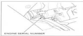
The engine serial number is stamped on the rear half of the lower crankcase, viewed from the right side.
