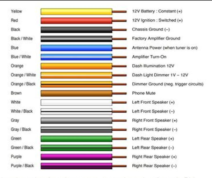
The color codes used on aftermarket car stereo connector harness's conform to the E.I.A (Electronics Industry Association) standards. These colors often differ from the wiring colors used by vehicle manufacturers. Always refer to your stereo owner's manual for specific wiring details before making any connections.
