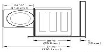
To ensure sufficient clearance for water lines and airflow, allow minimum clearances of at least 1 in. (2.5 cm) at the sides and 4 in. (10 cm) behind the unit. Be sure to allow for wall, door, or floor moldings that may increase the required clearances.
